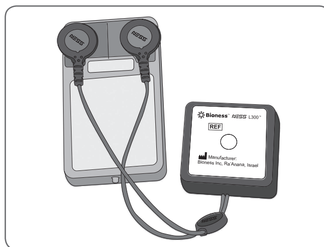
Figure 87: L300 Tester connected to the RF Stim Unit.
